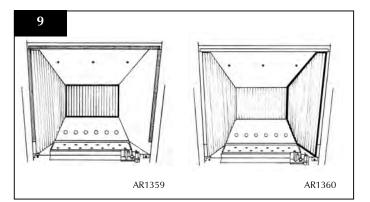
• Locate the top panel on top of the sides and rear by lifting it up and forward inside the box
